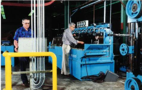
The wire rolling mill is used for sizing large diameter clad wire. It creates less work hardening than drawing, therefore reducing the number of anneals. Rolling also provides an excellent metallurgical bond between the core wire and the copper cladding.
