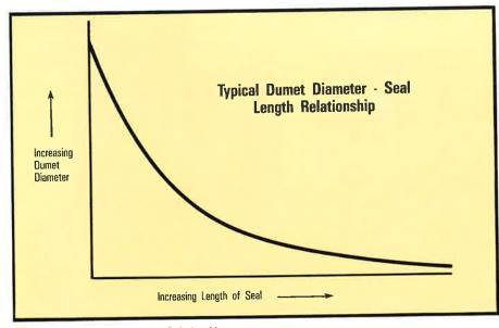
Figure 2 - Diameter/Seal Length Relationships
