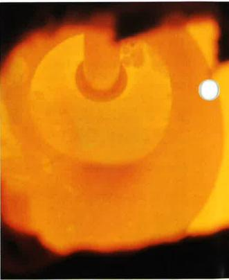
In the crucible, copper is metallurgically bonded to the care rod.
